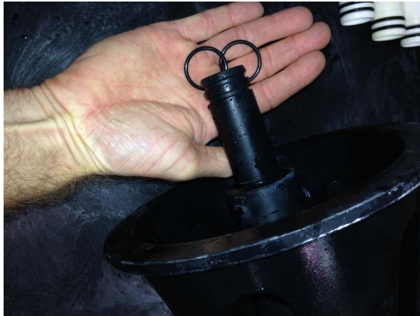
Figure 4.8 O-rings Removed from RO Pressure Vessel
