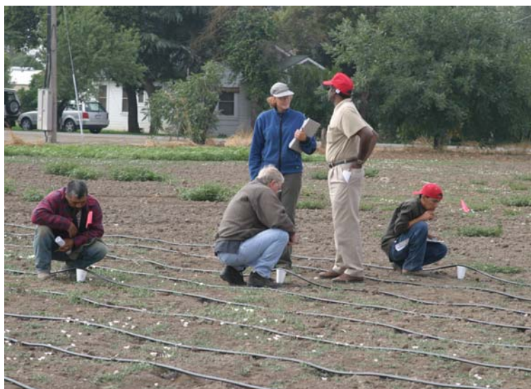
Participants check drip system distribution uniformity at the District's annual "fertigation" workshop, which is an agricultural technique of applying fertilizer through an irrigation system.
