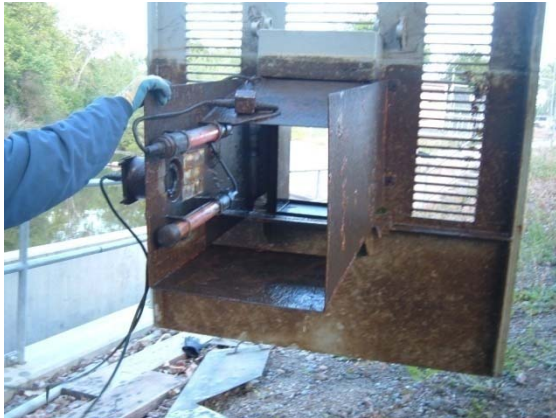
Figure 6. Masson Fishway deployment 2006-2008 Note flow through weirs on sides and metal extension collar to direct fish past the camera
