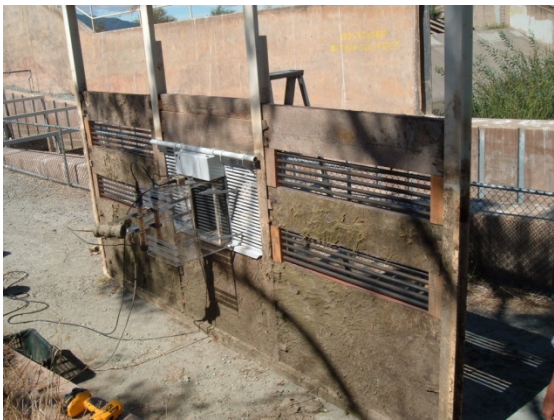
Figure 5. Alamitos Fishway deployment 2004-2006 Note larger flow through weirs and plexiglass extension
