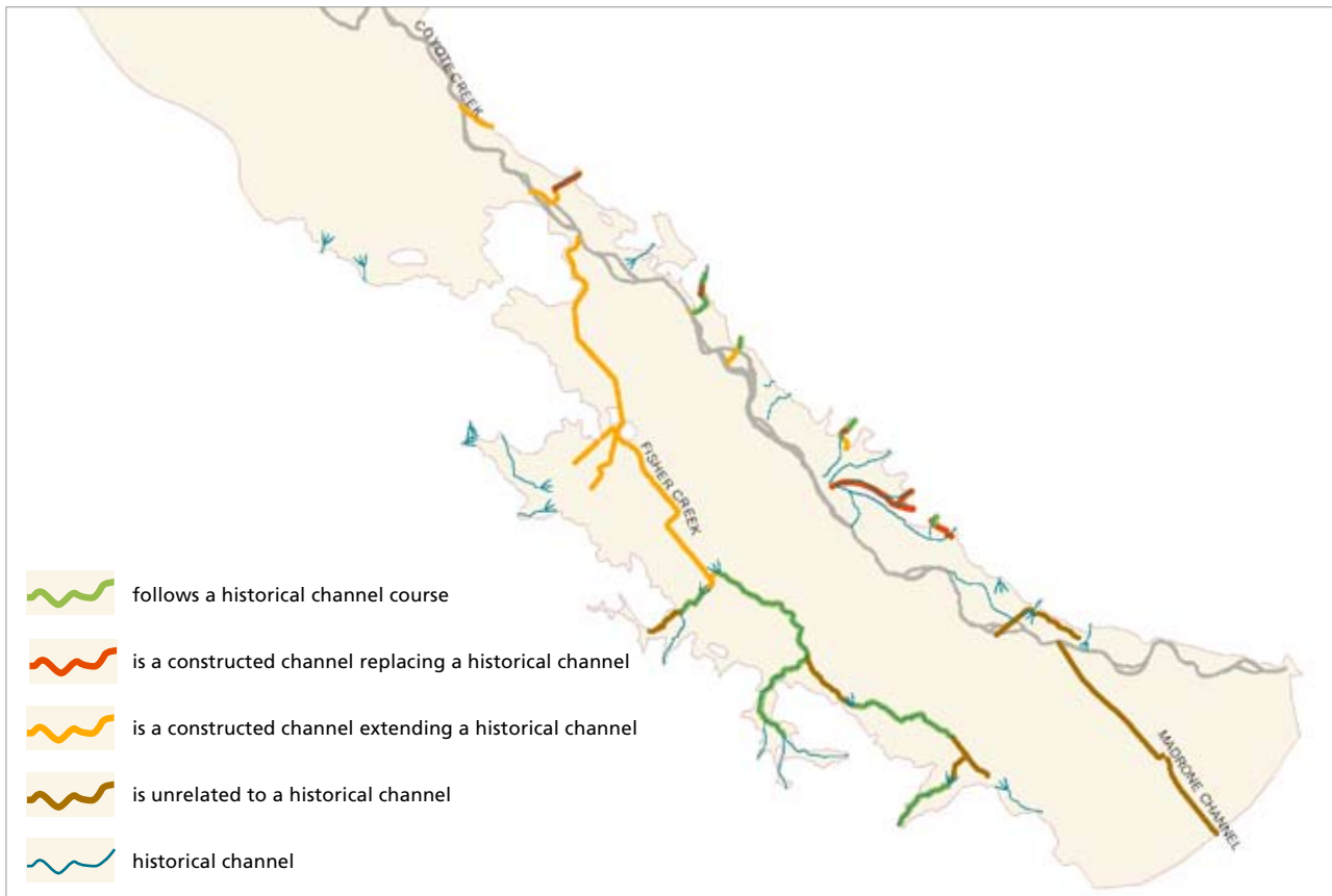
FIGURE IV-7B. ORIGIN OF MODERN CREEKS TRIBUTARY TO COYOTE CREEK (TOP). Nearly two thirds of the tributary drainage network on the valley floor is artificial channel, mostly created to extend discontinuous creeks to the Coyote mainstem.
