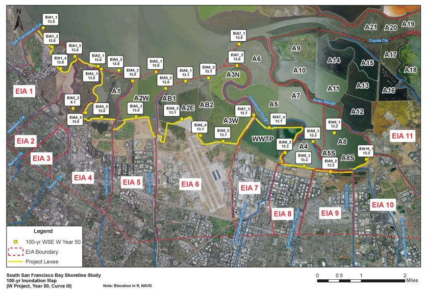
Figure 18. 100-year WSE under With Project Condition in Year 50 SLR Curve III
