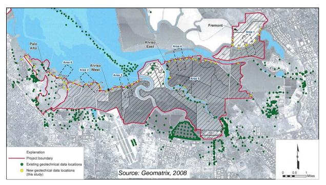
Figure 6. Geotechnical Exploration Map for Outer Levees
