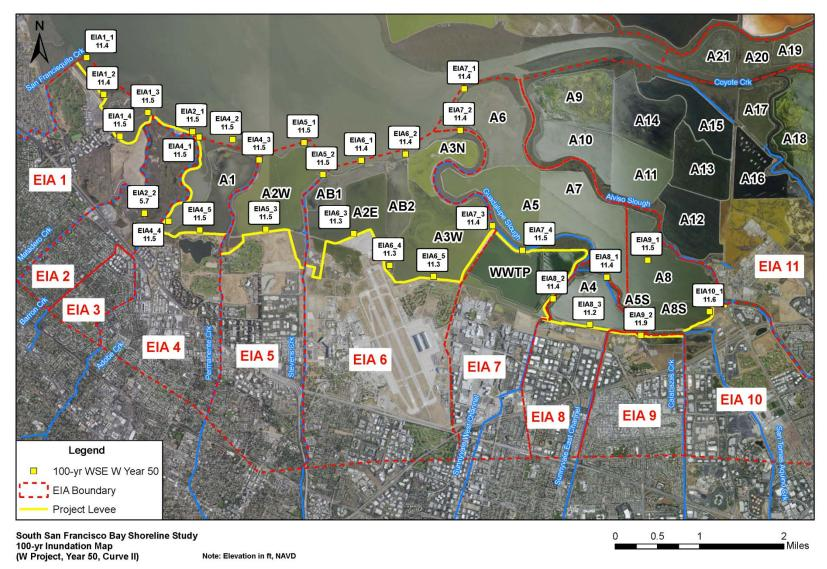
Figure 17. 100-year WSE under With Project Condition in Year 50 SLR Curve II
