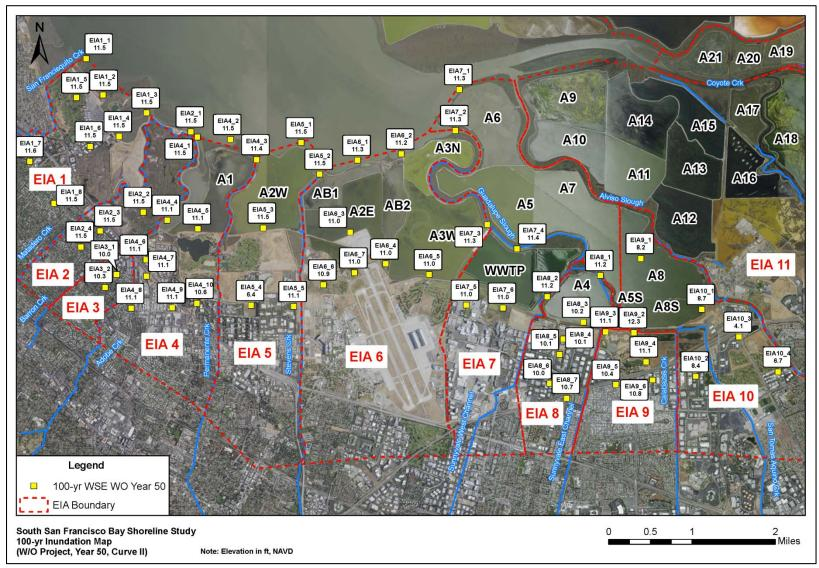
Figure 13. 100-year WSE under Without Project Condition in Year 50 SLR Curve II
