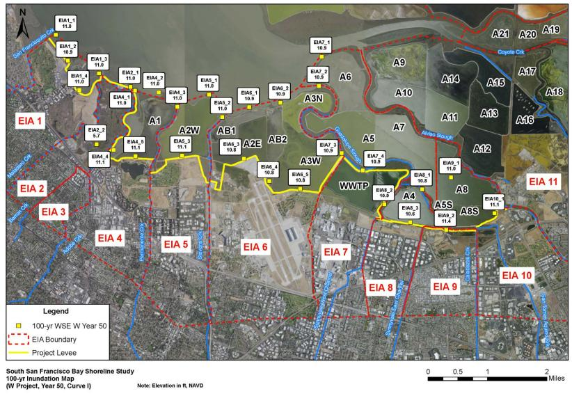
Figure 16. 100-year WSE under With Project Condition in Year 50 SLR Curve I
