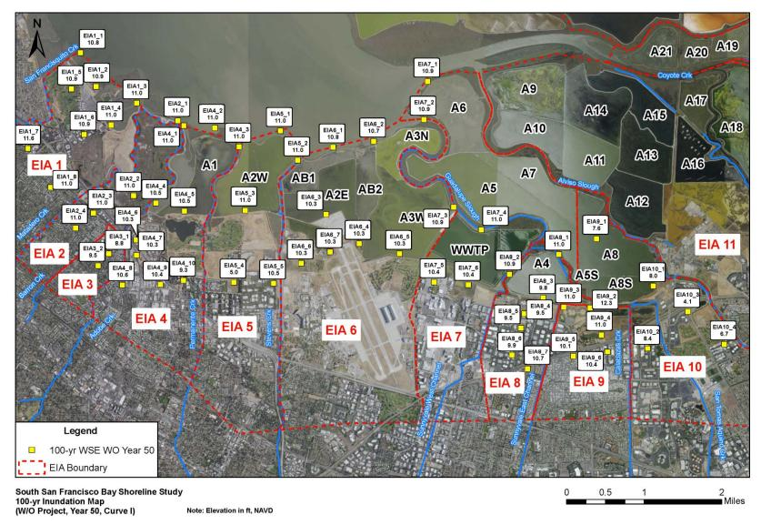
Figure 12. 100-year WSE under Without Project Condition in Year 50 SLR Curve I
