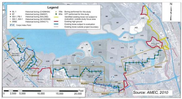
Figure 7. Geotechnical Exploration Map for Inner Levees
