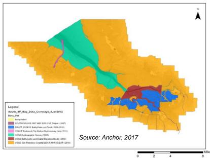
Figure 4. Data Sets Used to Generate A High Resolution of DEM
