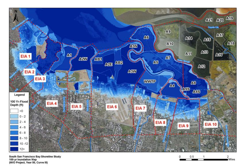
Figure 22. 100-year Inundation Map Without Project in Year 50 SLR Curve III
