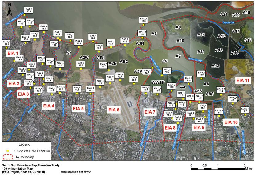
Figure 14. 100-year WSE under Without Project Condition in Year 50 SLR Curve III
