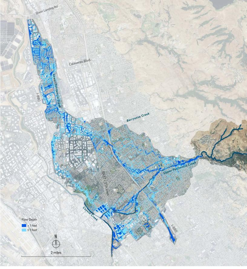
Modeled Upper Penitencia Creek Flow Contribution to Flooding on the Valley Floor. Modeling shows the flooding extent in the urbanized valley floor (blue) around Upper Penitencia Creek for a 100-year flood event. Modeling results courtesy of the Santa Clara Valley Water District.
