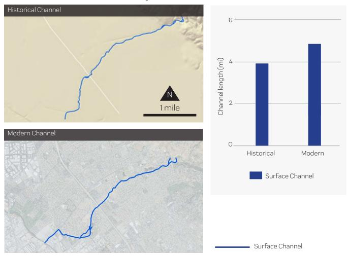
Historical and Modern Channel Planform. The overall channel planform has remained relatively unchanged between historical (mid-19th c.) and modern (early 21st c.) time periods, with the mainstem channel length increasing by approximately 1 mile.
