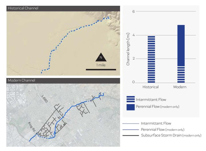
Historical and Modern Stream Flow Patterns. Much of Upper Penitencia Creek now has perennial flow during most years, though areas in the middle reaches still have intermittent flows. Storm drains now carry runoff directly to the creek.
