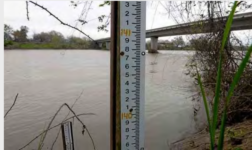
Example of a water height stage indicator.
