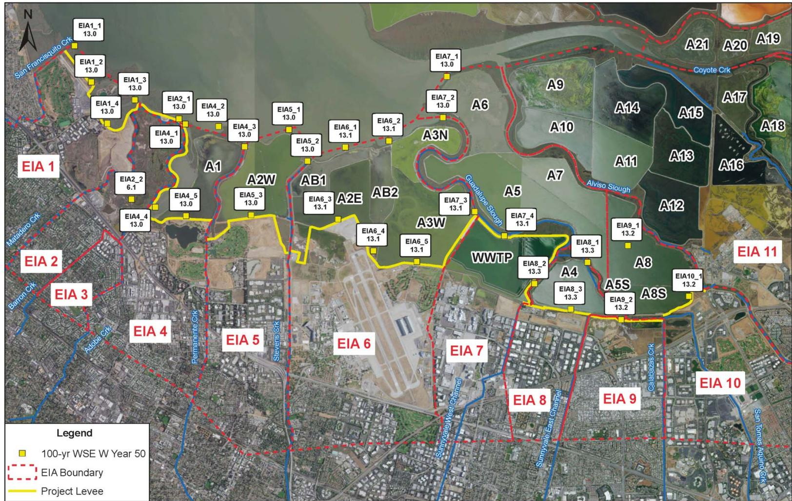
Figure 18. 100-year WSE under With Project Condition in Year 50 SLR Curve III
