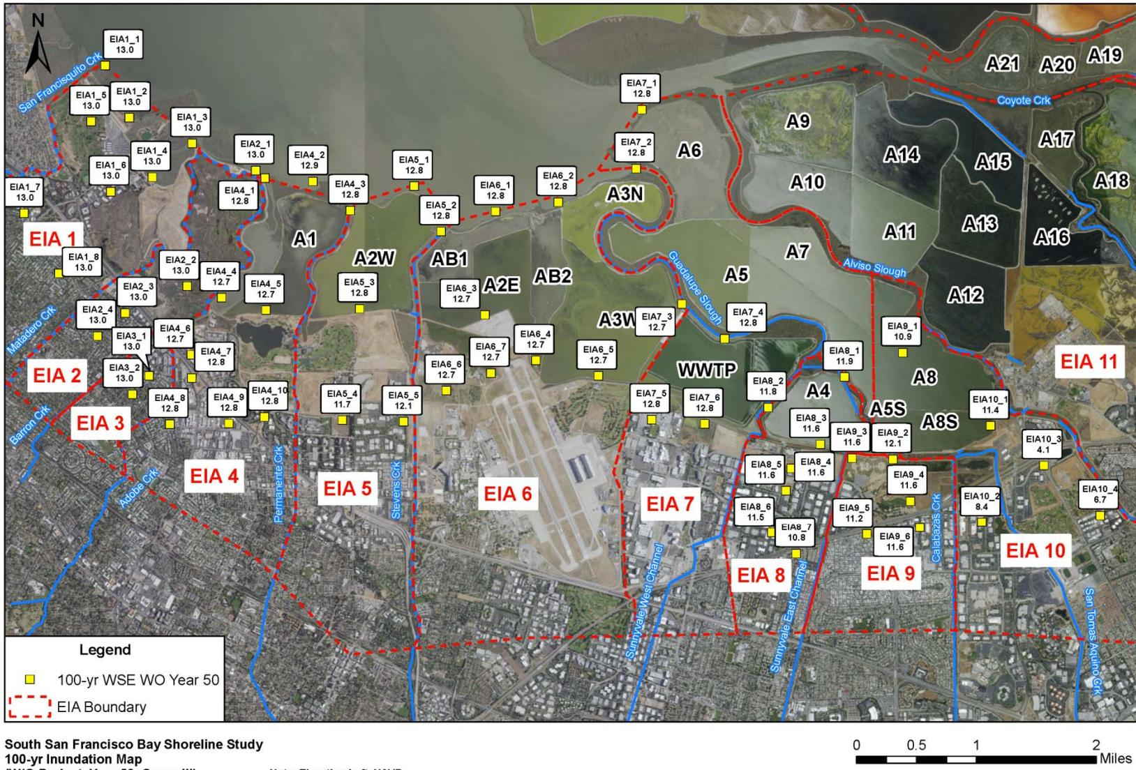
Figure 14. 100-year WSE under Without Project Condition in Year 50 SLR Curve III
