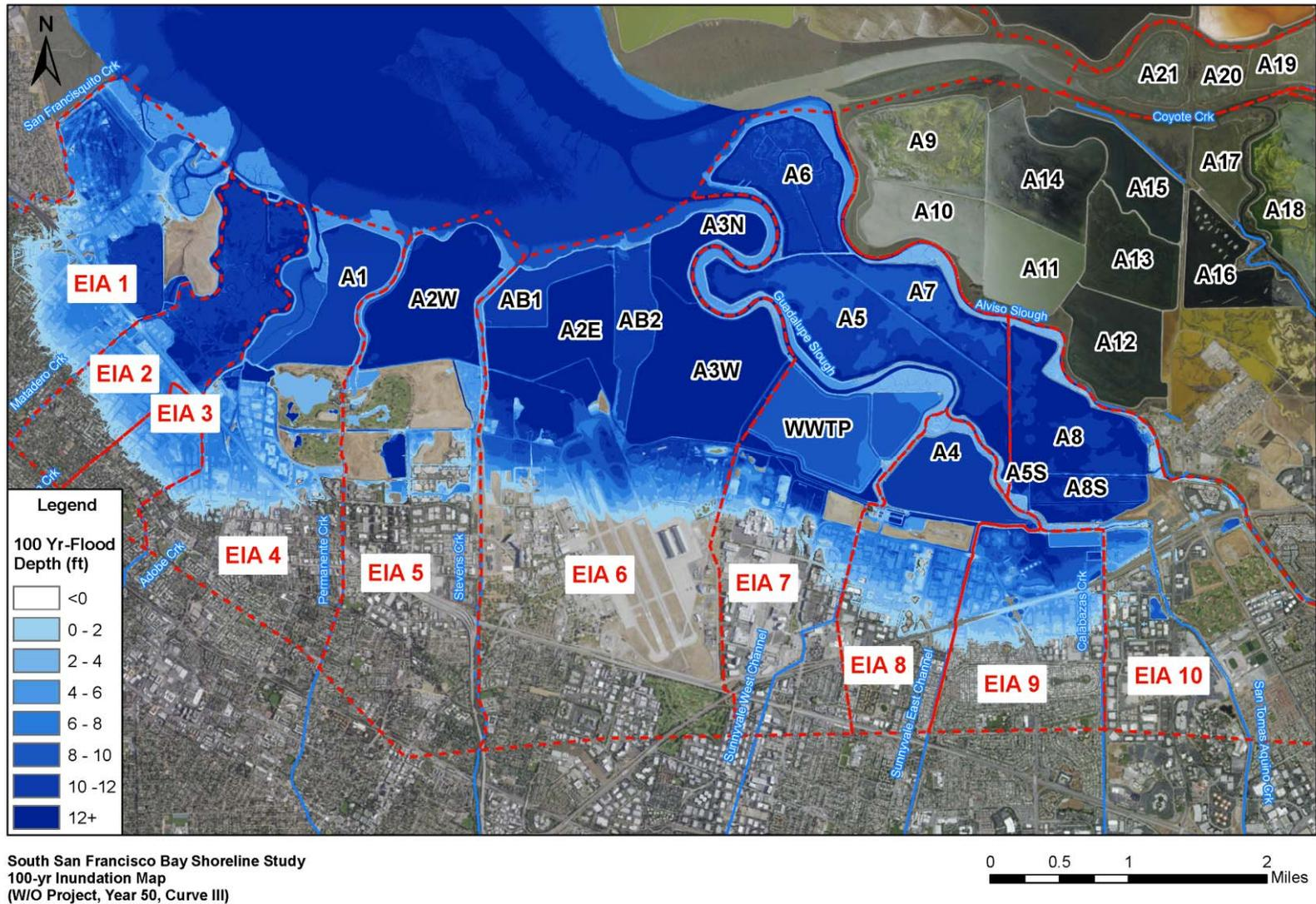
Figure 22. 100-year Inundation Map Without Project in Year 50 SLR Curve III
