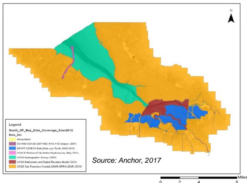
Figure 4. Data Sets Used to Generate A High Resolution of DEM
