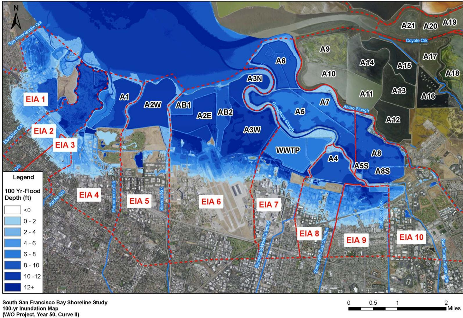
Figure 21. 100-year Inundation Map Without Project in Year 50 SLR Curve II
