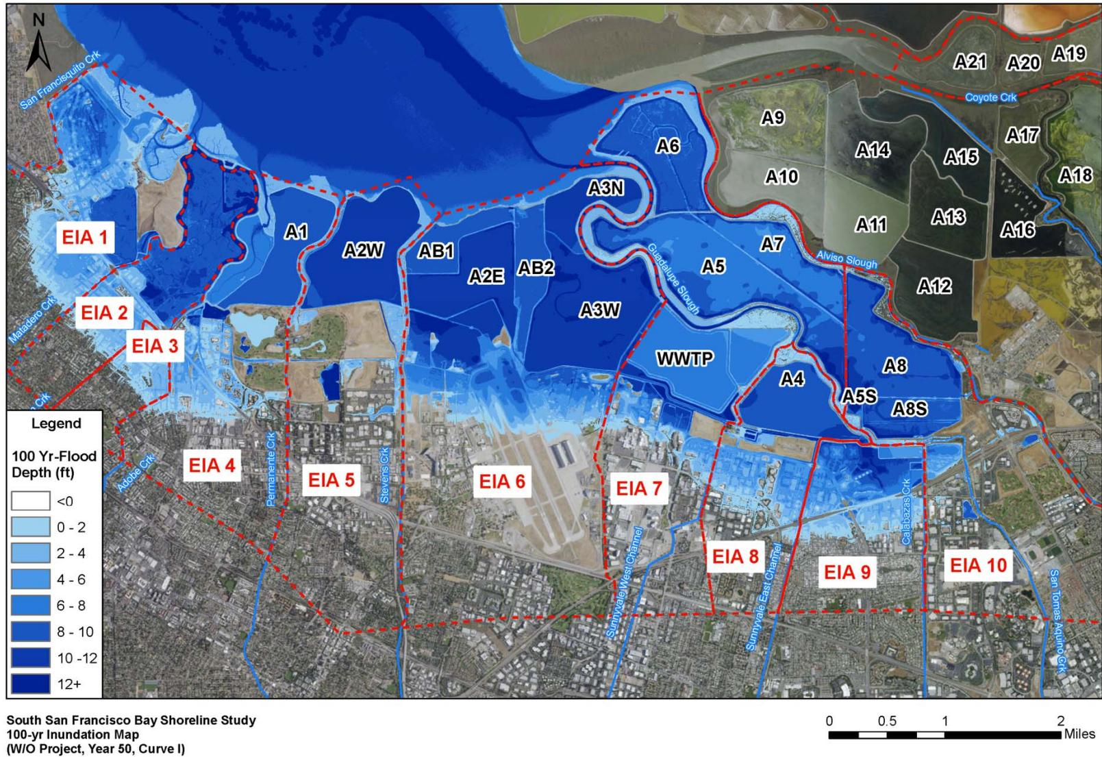
Figure 20. 100-year Inundation Map Without Project in Year 50 SLR Curve I
