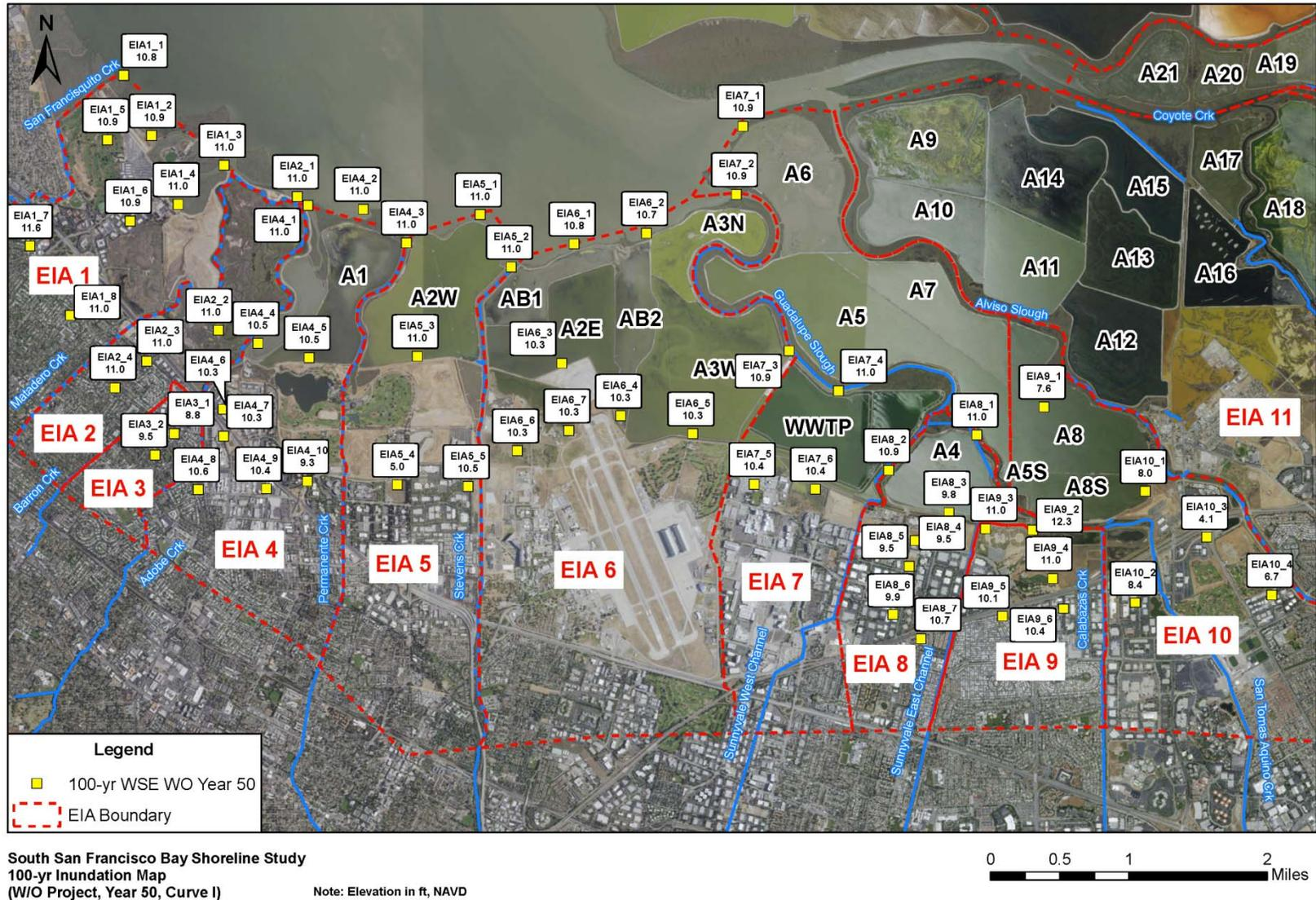
Figure 12. 100-year WSE under Without Project Condition in Year 50 SLR Curve I
