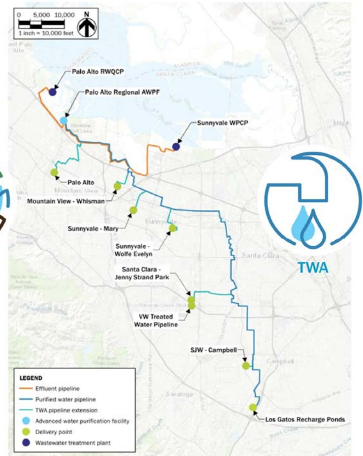
Figure 9-7. Flexible implementation from San José-based AWP: TWA Flex facility locations and pipeline alignments
