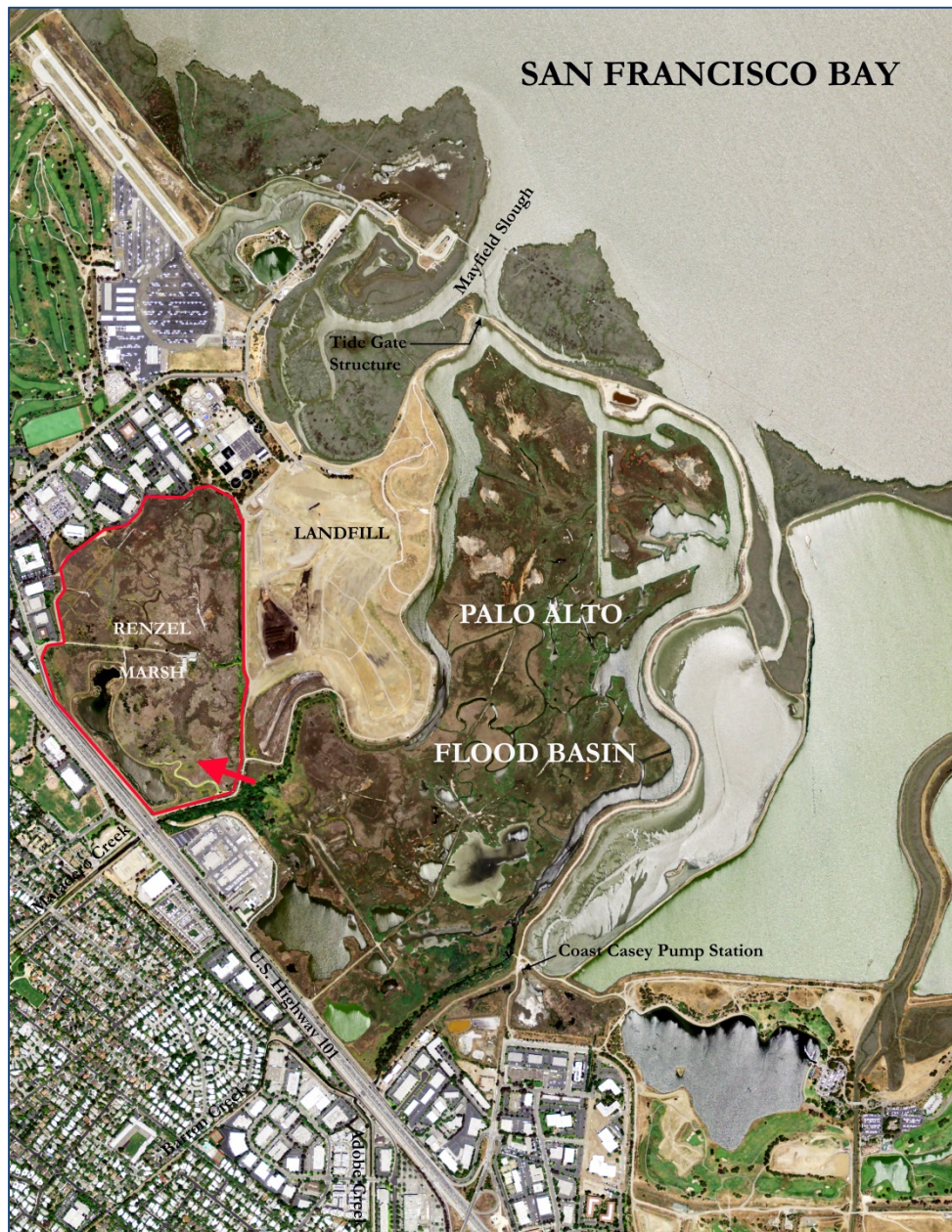
Figure 31. Overflow to Renzel Marsh to Create Additional Storage
