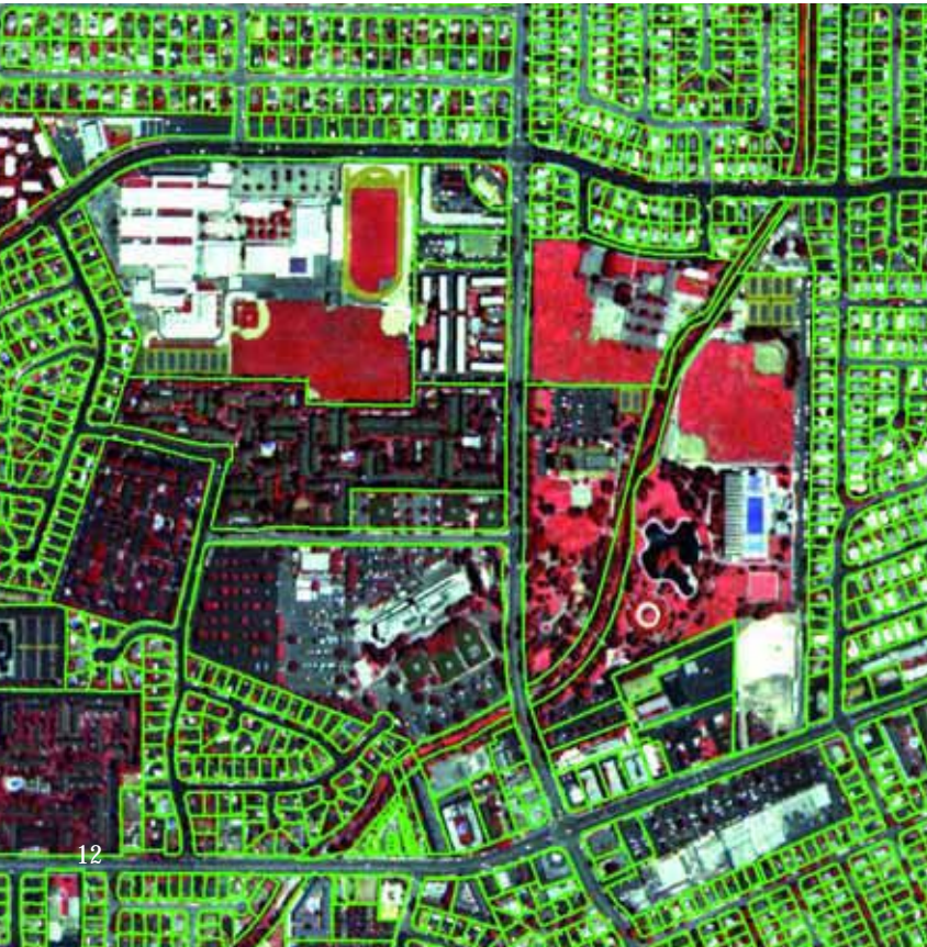
Multi-spectral images were used to develop "classification layers" which identify different types of groundcover.
