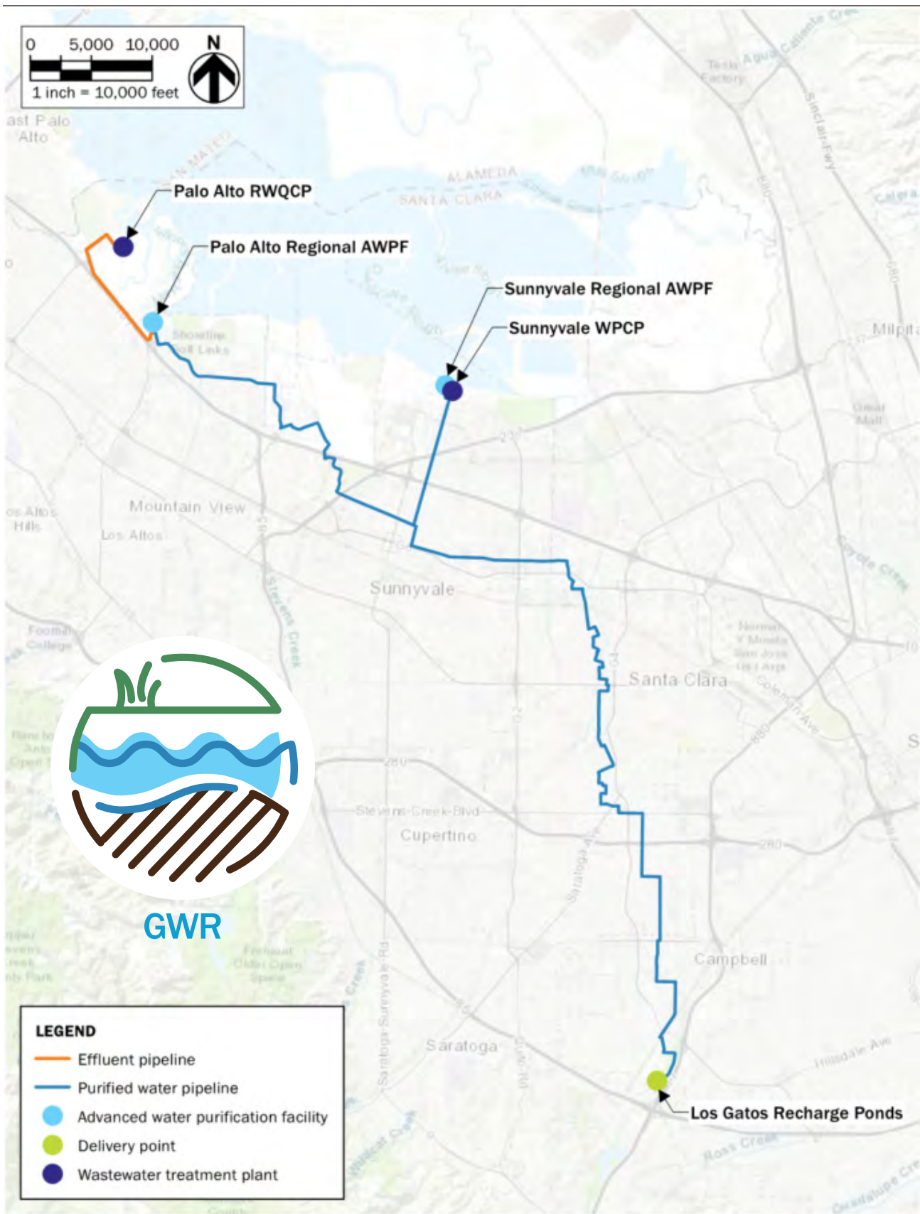
Figure 6-7. Portfolio 4: PA/SV GWR facility locations and pipeline alignments
