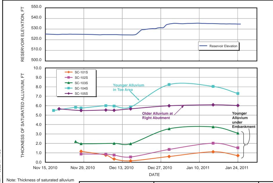
as measured in Casagrande piezometers installed in sonic borings.
