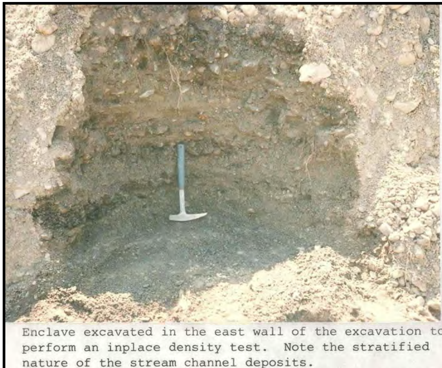
Photo 4 - Younger alluvium exposed in excavation for outlet modifications (DSOD / L.Y. Dudley, June 1985)
