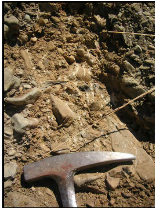
Photo 8 - Santa Clara Formation conglomerate (clayey sand with gravel) exposed along Stevens Canyon Road cut on left side of reservoir (300 ft upstream from left end of dam)
