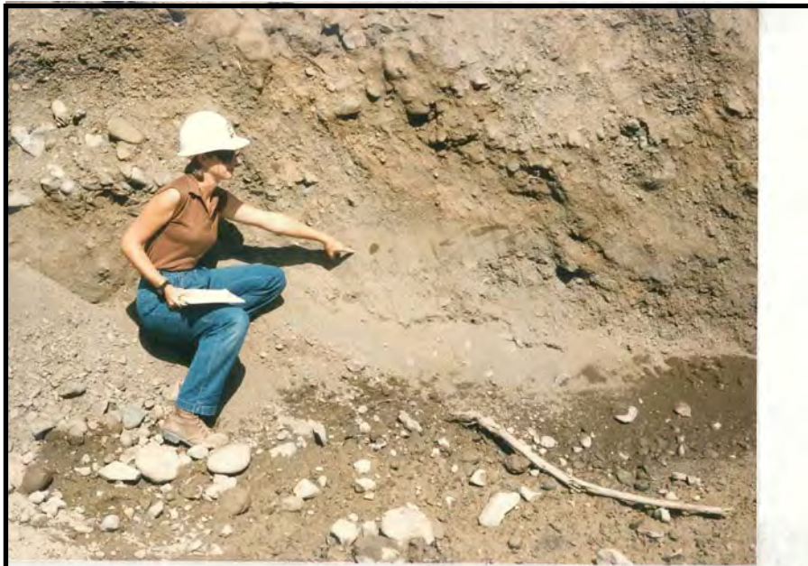
Stream channel deposits on the west side of the excavation showing a cross-bedded, poorly graded sand lens.
