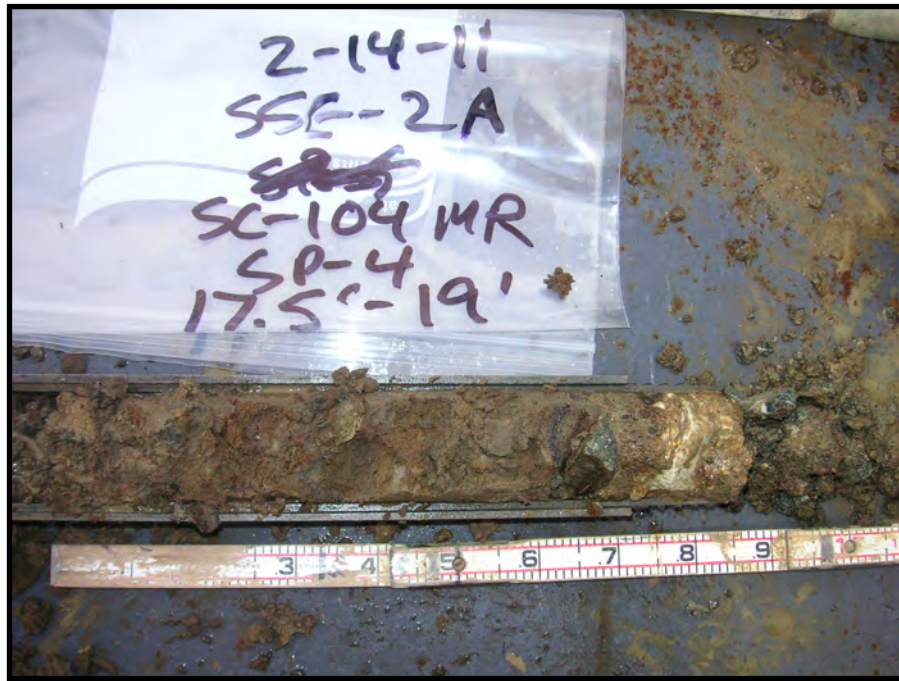
Photo 3 - Layer of clayey sand with gravel in uppermost younger alluvium SC-104 MR ~17-18.2 ft (left/upper 0.7 ft of sampler)
