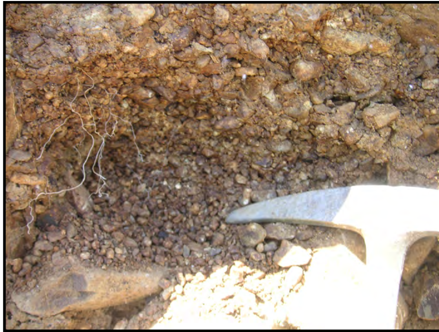
Photo 7 - Gravelly sand terrace alluvium exposed along left bank of reservoir near high water line (immediately north of boat ramp)
