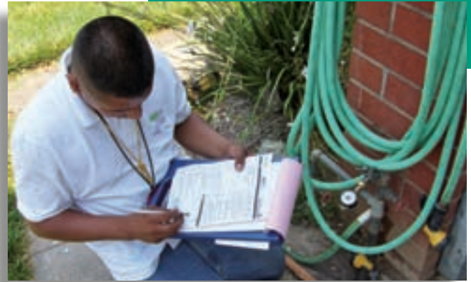
Checking the water pressure during a Water-Wise House Call.
