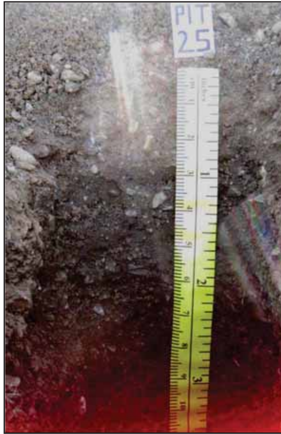
Figure 71: Soil Profile Description Location 25.1 in reach 7a - A picture depicting the massive, man modified fill that keys out as a Sandy-skeletal, mixed, Typic Xerofluvent (the closest taxonomic analog)
