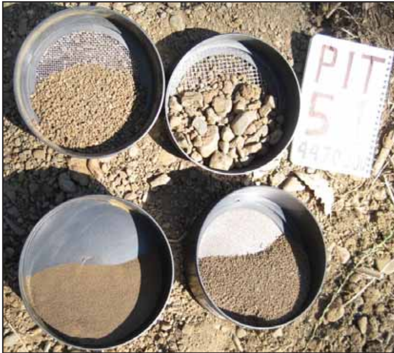
Figure 17: Soil Profile Description and Sampling Location 5.1 in Reach 4 - A picture depicting the proportional soil textural separates. (The soil was sampled from the top 20 inches of a profile located on the left mid-terrace flank of the creek, looking downstream)
