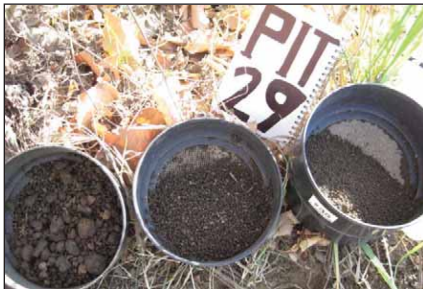
Figure 84: Soil Profile Description and Sampling Location 29.1 in Reach 7b - A picture depicting the differing ped sizes, structure and color. The soil was sampled from the top 20 inches of the profile.
