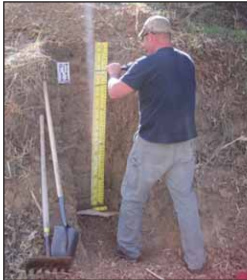
Figure 2: Soil Profile Description Location 1.1 in Reach 4 - A picture depicting the use of a static cone penetrometer (and a hand-held geotester) to quantifiably assess the topsoil's strength and the depth to densic materials.
