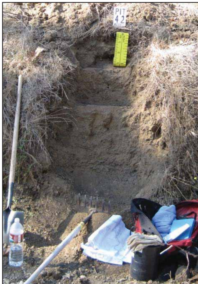
Figure 14: Soil Profile Description Location 4.2 in Reach 4 - A picture depicting the soil profile of a Coarse-loamy, mixed, thermic Typic Haploxeralf. The soil profile was positioned to examine the material that forms the terrace embankment down to the bottom of the channel invert. The profile was located on the right side of the creek, looking downstream.
