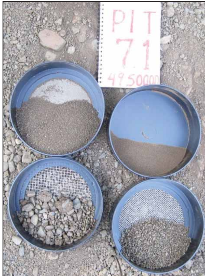
Figure 22: Soil Profile Description Location 7.1 in Reach 4 - A picture depicting the proportional soil textural separates. The soil was sampled from the top 20 inches of a profile that forms the right terrace embankment.
