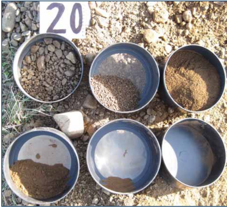
Figure 59: Soil Profile Description and Sampling Location 20.1 in Reach 6a - A picture depicting the proportional soil textural separates. The soil was sampled from the top 20 inches of the profile.
