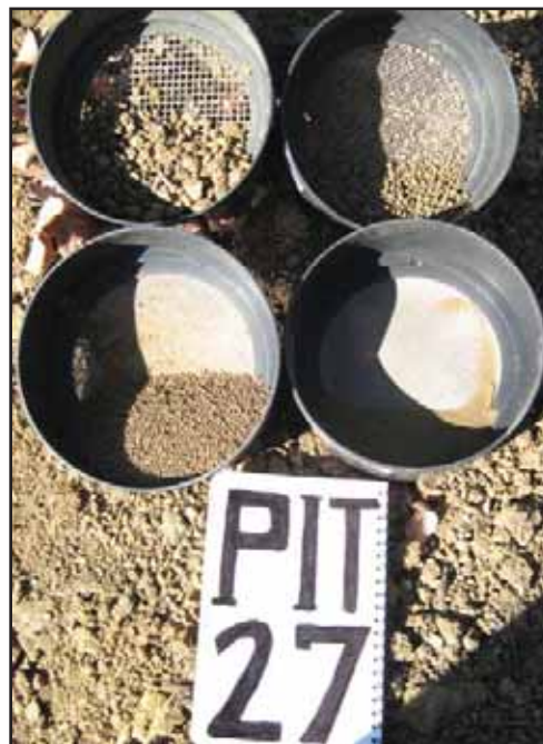
Figure 78: Soil Profile Description and Sampling Location 27.1 in Reach 7b - A picture depicting the proportional soil textural separates. The soil was sampled from the top 20 inches of the profile.
