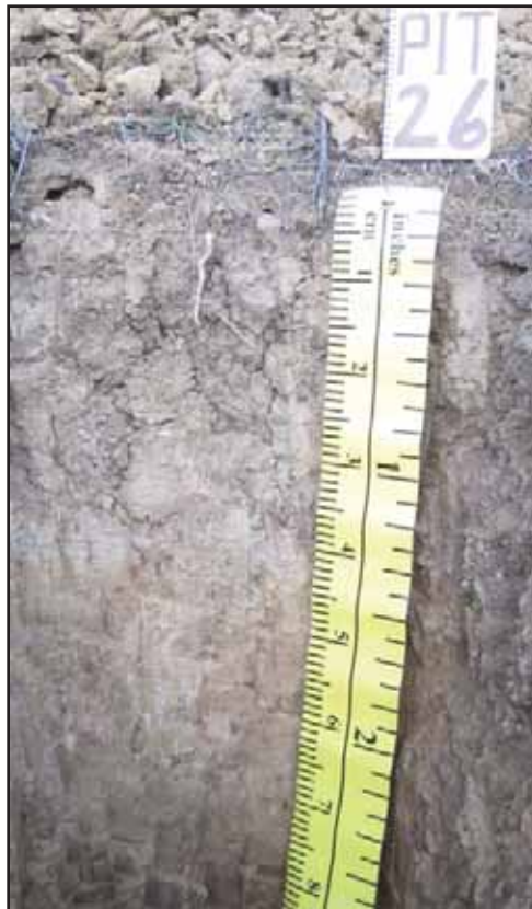
Figure 74: Soil Profile Description Location 26.1 in Reach 7b - A picture depicting the massive man modified fill - soil profile that keys out as a Coarse-loamy, mixed, thermic Typic Haploxeralf. The soil profile examined the soil material from the middle of the road embankment down to the bottom of the engineered channel invert. The soil profile pit was positioned on the left side of the channel, looking southwest (downstream).
