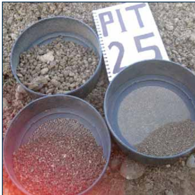
Figure 72: Soil Description and Sampling Location 25.1 in Reach 7a - A picture depicting the proportional soil textural separates. The soil was sampled from the top 20 inches of the profile.
