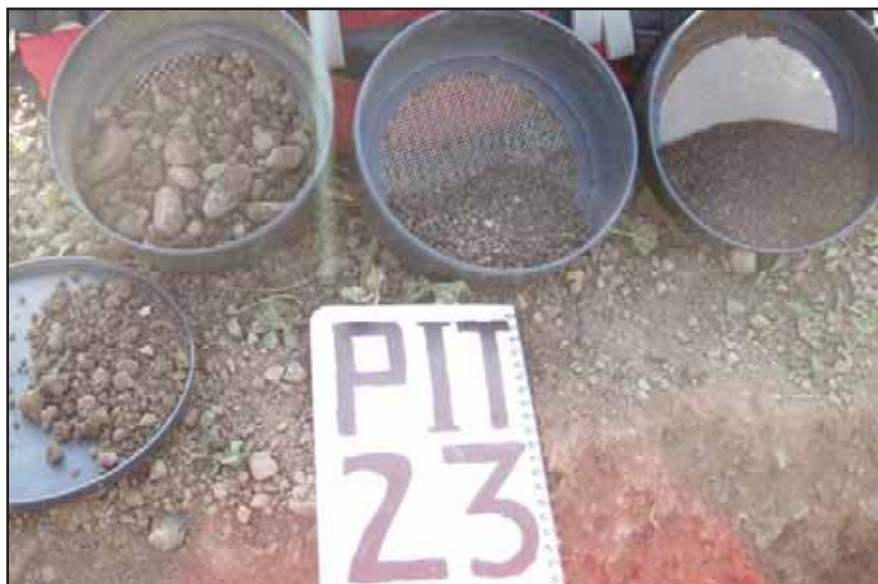
Figure 66: Soil Profile Description and Sampling Location 23.1 in Reach 7a - A picture depicting the proportional soil textural separates. The soil was sampled from the top 20 inches of the profile.
