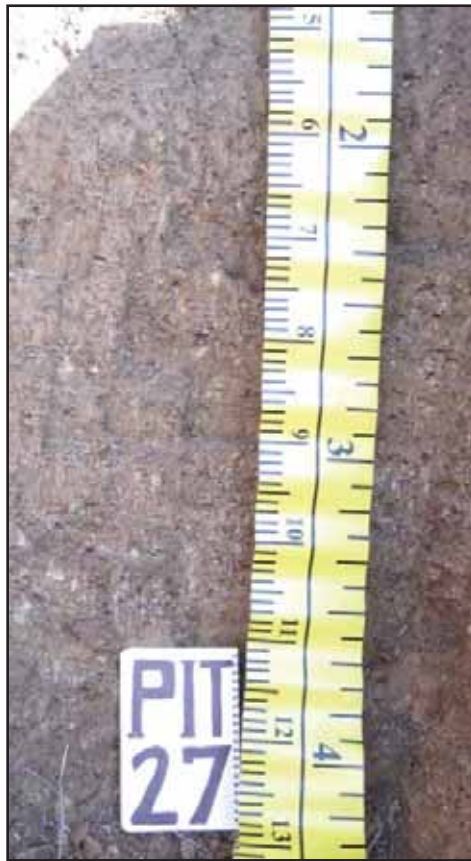
Figure 77: Soil Profile Description Location 27.1 in Reach 7b - A picture depicting the massive embankment fill that keyed out as a man-modified Loamy-skeletal, mixed, thermic Typic Xerorthent.
