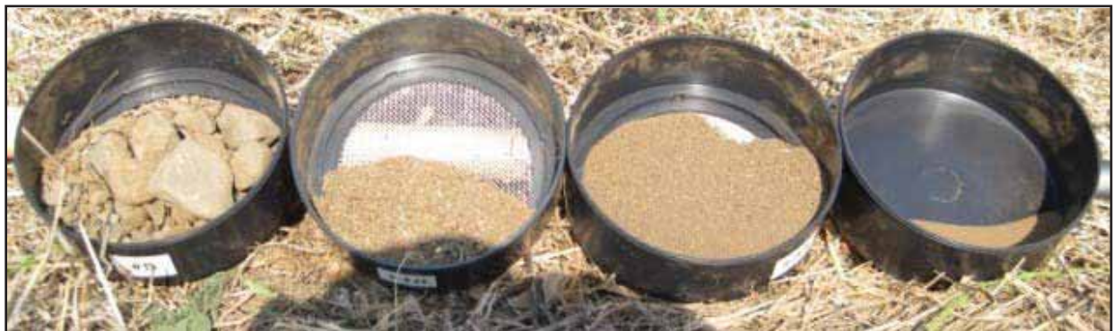
Figure 30: Soil Profile Description and Sampling Location 10.1 in Reach 5 - A picture depicting the proportional soil textural separates. (The soil was sampled from the top 20 inches of a profile located on the left mid-terrace flank of the creek, looking downstream)
