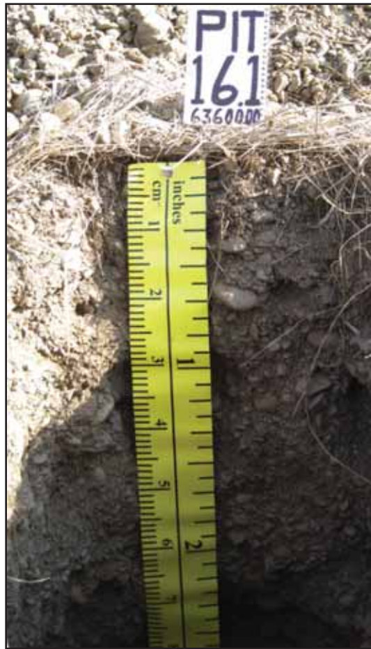
Figure 45: Soil Profile Description Location 16.1 in Reach 6b - A picture depicting the upper part of the soil profile of a Loamy-skeletal, mixed, Typic Xerofluvent. The soil profile was positioned on a mid-terrace flank located on the left side of the creek, looking downstream.
