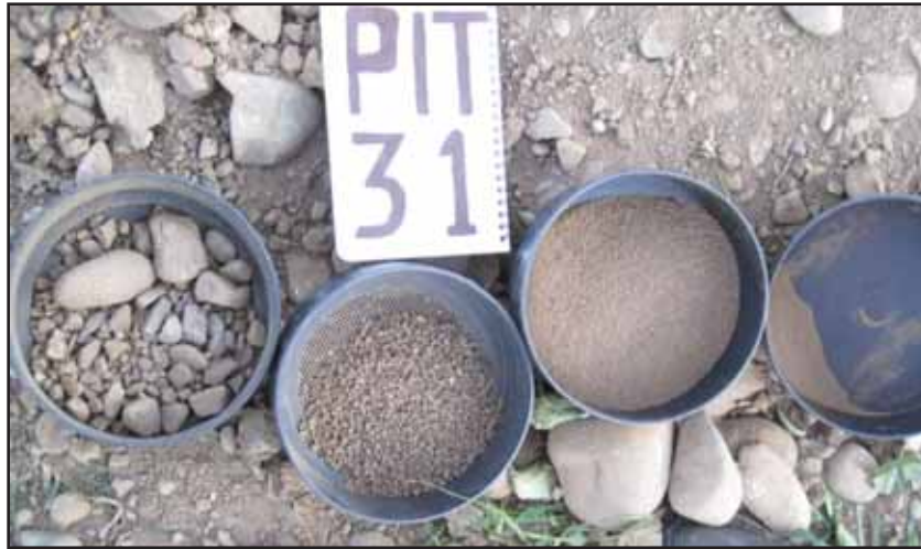
Figure 89: Soil Description Location 31.1 in Reach 14 - A picture depicting the proportional soil textural separates. The soil was sampled from the top 20 inches of the profile.
