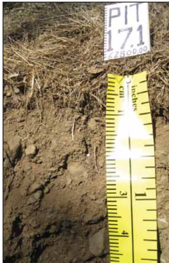
Figure 48: Soil Profile Description Location 17.1 in Reach 6b - A picture depicting the upper part of the soil profile of a Loamy-skeletal, mixed, thermic Typic Xerorthent. The soil profile was positioned on a mid-terrace flank located on the left side of the creek, looking downstream.
