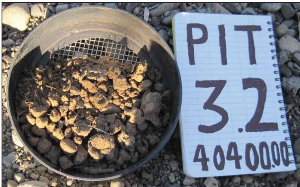
Figure 10: Soil Profile and Sampling Description Location 3.2 - A picture depicting size, shape, and type of ped structure. (The soil was sampled from the top 20 inches of a profile that forms the right terrace embankment)
