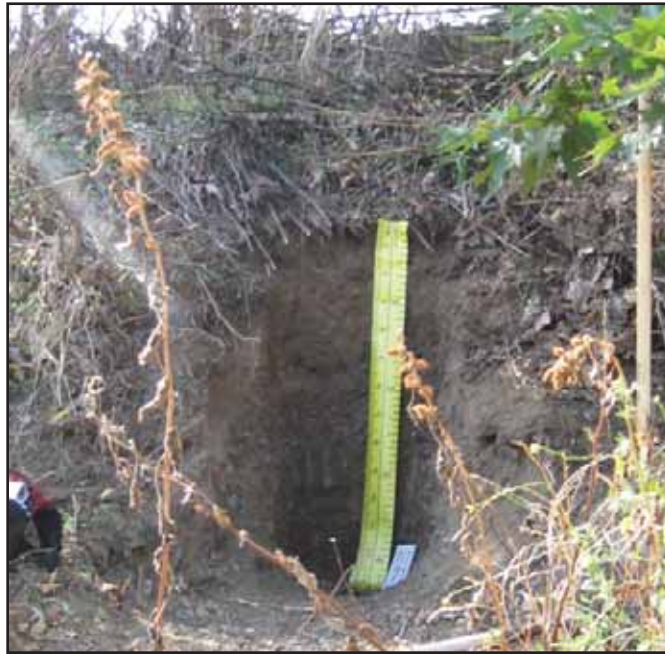
Figure 21: Soil Profile Description Location 7.1 in Reach 4. - A picture depicting the soil profile's location. The soil profile was positioned to examine the material that forms the terrace embankment down to the bottom of the channel invert. The soil profile was located on the right side of the creek, looking downstream.
