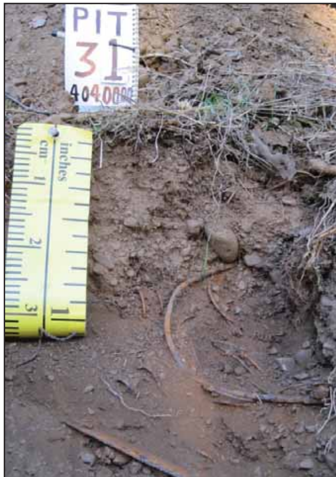
Figure 8: Soil Profile Description Location 3.1 in Reach 4 - A picture depicting the soil profile being comprised of manmade fill and debris, This soil classified as a Loamy-skeletal, mixed, thermic Typic Xerofluvent (Man-Modified). (The soil profile was positioned on a mid-terrace flank located on the left side of the creek, looking downstream)
