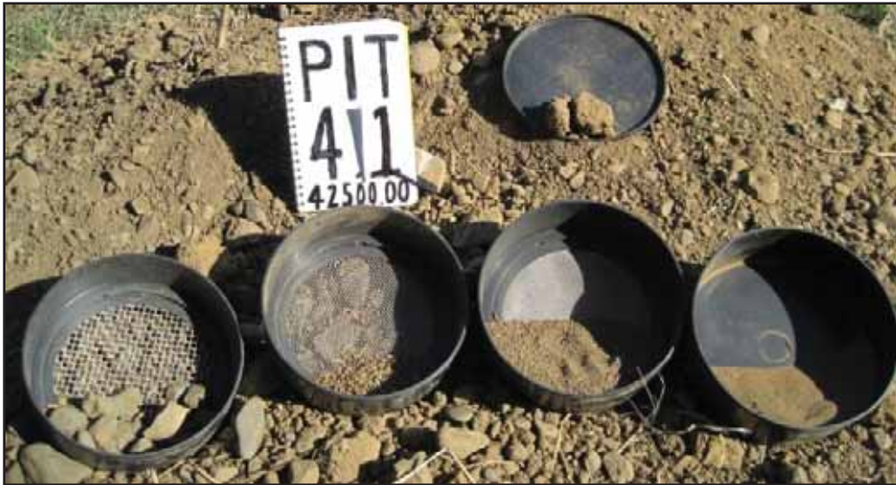
Figure 13: Soil Profile Description and Sampling Location 4.1 in Reach 4 - A picture depicting the proportional soil textural separates and ped structure. The soil was sampled from the top 20 inches of a profile located on the left mid-terrace flank of the creek, looking downstream.
