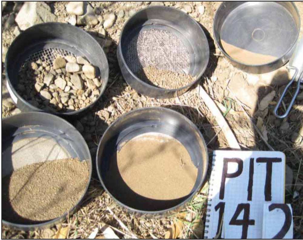
Figure 39: Soil Profile Description and Sampling Location 14.2 in reach 6b - A picture depicting the proportional soil textural separates. The soil was sampled from the top 20 inches of a profile located on the right mid-terrace flank of the creek, looking downstream.
