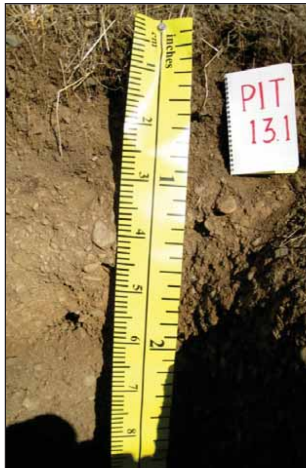
Figure 34: Soil Profile Description Location 13.1 in Reach 6b - A picture depicting the soil profile of a Loamy-skeletal, mixed, thermic Typic Xerorthent. The soil profile was positioned on a mid-terrace flank located on the left side of the creek, looking downstream.
