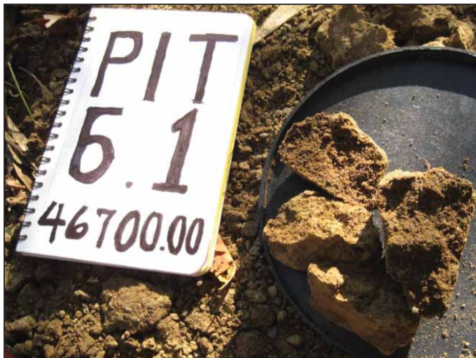
Figure 20: Soil Profile Description and Sampling Location 6.1 in Reach 4 - A picture depicting the medium to coarse subangular blocky structure and the interior ped face color. The soil was sampled from the top 20 inches of a profile that forms the right terrace embankment
