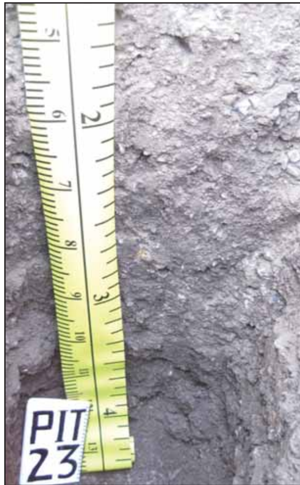
Figure 65: Soil Profile Description Location 23.1 in Reach 7a - A picture depicting the lower part of the soil profile of a Loamy-skeletal, mixed, Typic Xerofluvent.
