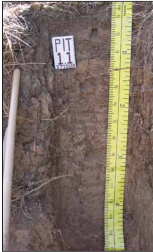
Figure 1: Soil Profile Description Location 1.1 in Reach 4 – A picture depicting the soil profile of a Coarse-loamy, mixed, thermic Typic Haploxeralf. The soil profile was located north of Buena Vista Avenue at the southern boundary of the Project Area. (The soil profile was positioned to examine the material that forms the terrace embankment down to the bottom of the channel invert. The soil profile was located on the right side of the creek, looking downstream.)
