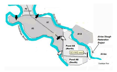
Removal of vegetation from the Slough will cause more water to be retained in the Slough and less will go over the Weir into Pond A8. The Slough past the Marina cannot handle that level of water. Additional flows would weaken downstream levees, and result in spill-over into Pond A12, which in turn would flood Alviso.
