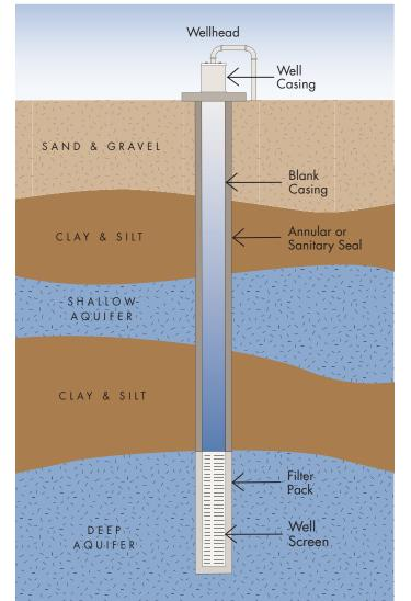
The typical domestic well in Santa Clara County is constructed by drilling a hole in the ground to a depth of 100 to 300 feet. As the well driller is drilling the hole, the type and depth of materials that the bit passes through are noted. This information is recorded on the driller log that is submitted to the permitting agency and provided to the well owner by their drilling contractor.
