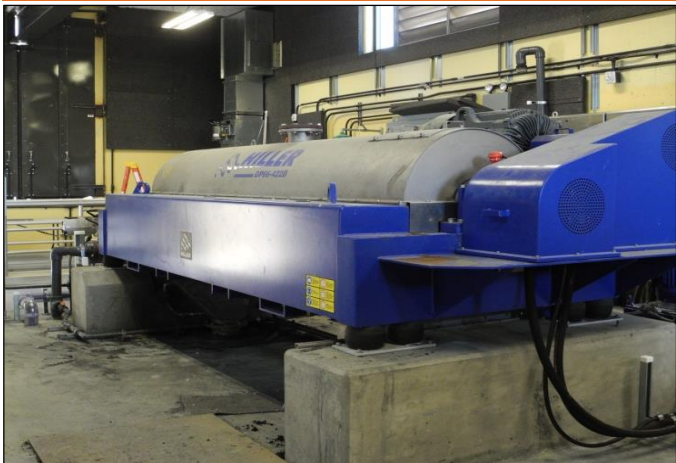
Centrifuge for mechanical dewatering of sludge
