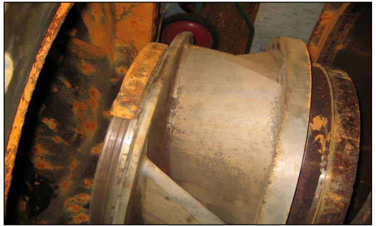
Example of bacterial corrosion on a suction wear ring of an impeller
