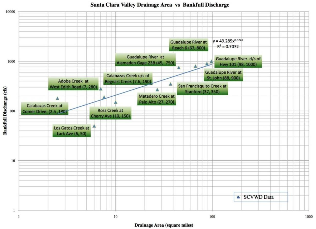
**Figure 6: Bankfull Discharge Versus Drainage Area SCVWD Regional Curve**
