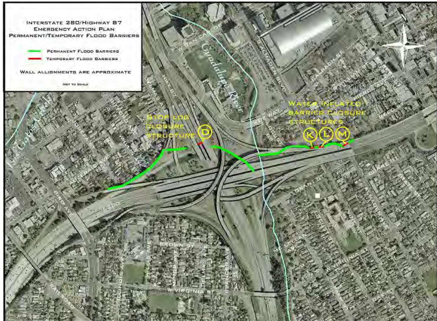
FIGURE 2B: Temporary Flood Barrier Locations
