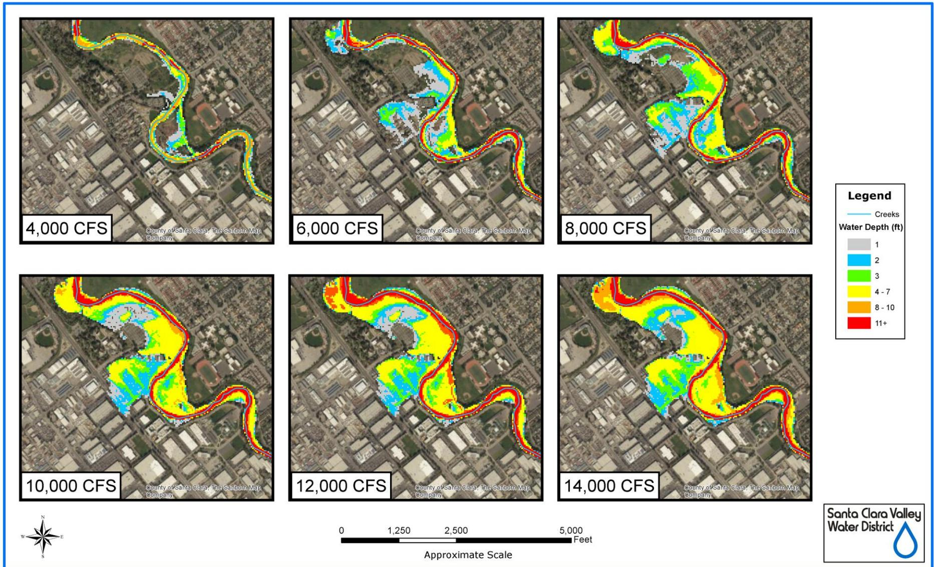
Figure 40: Rock Springs flood map (Pre-Rock Springs flood wall and berm project)
