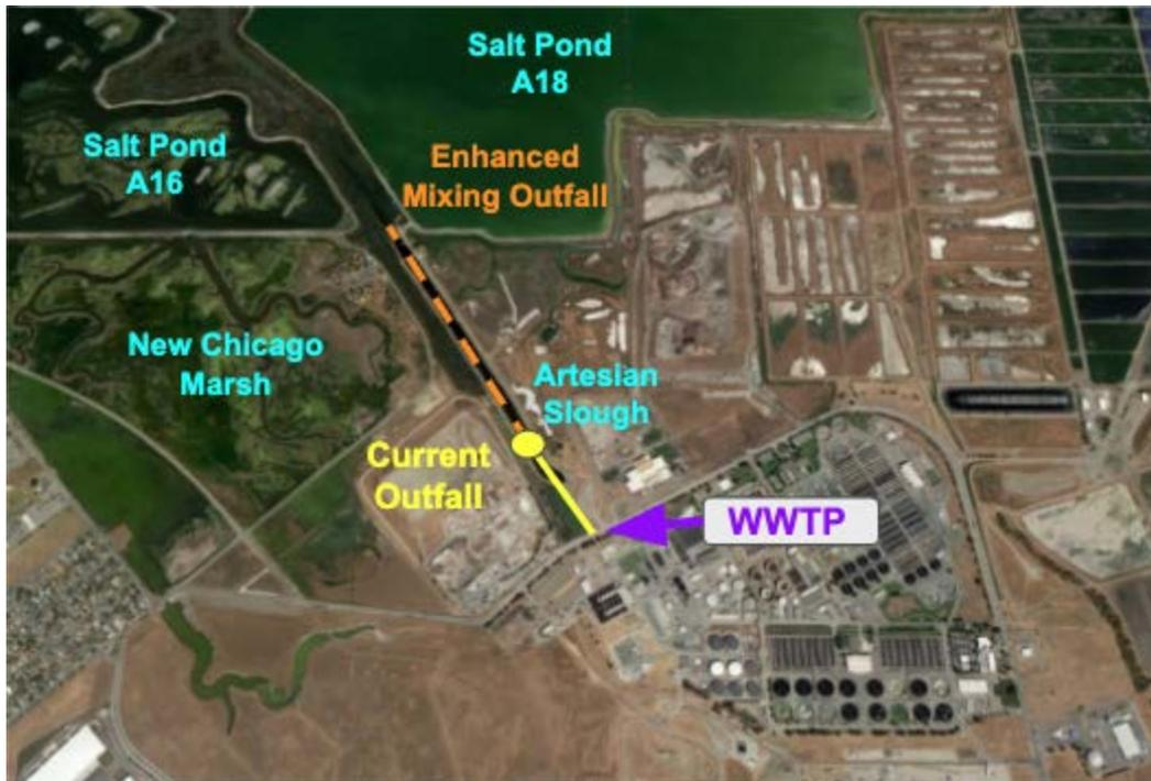
**Figure 13.** Current and New Enhanced Mixing Outfalls for the Wastewater Treatment Plant (WWTP) in San Jose Santa Clara as a part of Portfolio 1 Scenarios A and B (GHD Draft, 2019). Salinity is likely to decrease at the new outfall.
