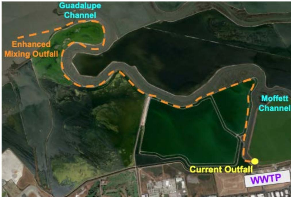
**Figure 14.** Current and New Enhanced Mixing Outfalls for the Wastewater Treatment Plant (WWTP) in Sunnyvale as a part of Portfolio 2 Scenario A and Portfolio 4 (GHD, 2019). Moving the current outfall may increase salinity in Moffett Channel.
