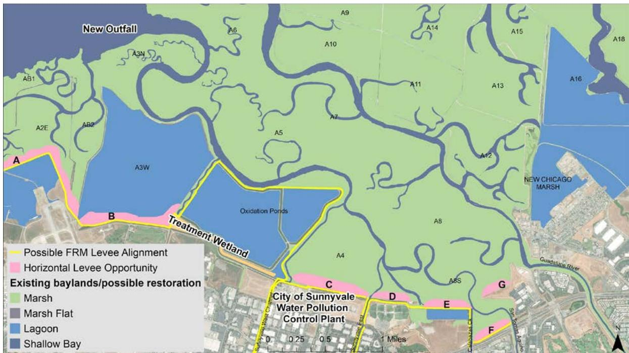
**Figure 9.** There are several potential locations (labeled A - G) in the immediate area of the Sunnyvale treatment plant where ROC could be discharged to a horizontal levee.
