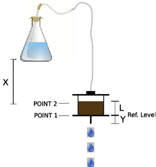
Figure 2.4: A diagram of a column/Mariotte apparatus used in the constant head method.
