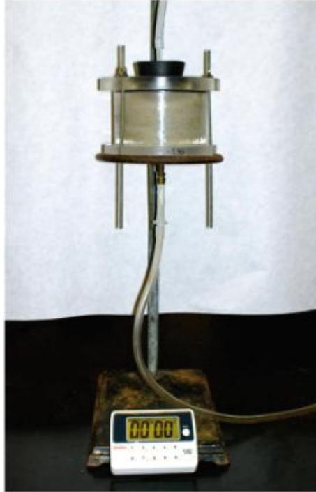
Figure 2.1: CO<sub>2</sub> saturation of a soil column.
