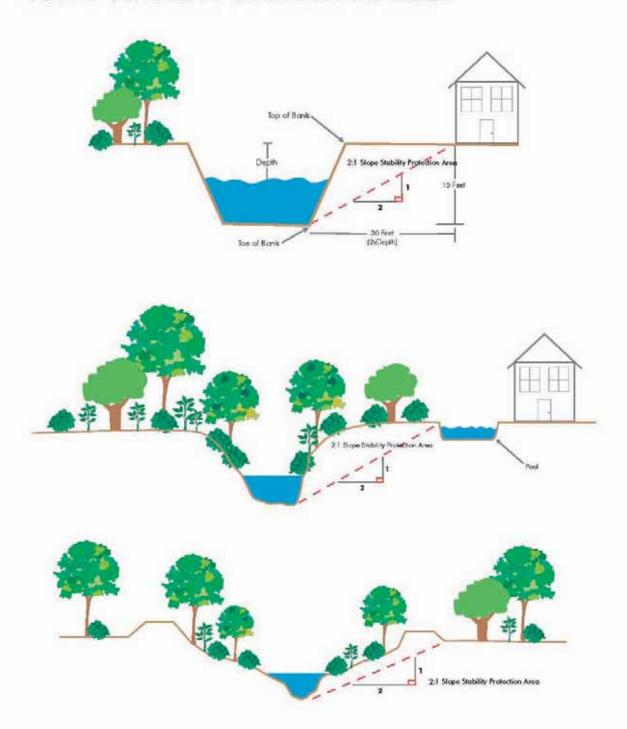
Note: While accessory structures are typically exempt, it is still recommended to locate them outside the 2:1 Slope Stability Protection Area in order to protect the structures, creek bank, and habitat.
